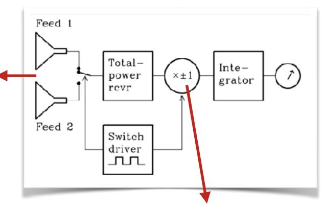
Output of receiver is **multiplied by +1** when receiver is connected to **feed 1 and by -1** when connected to **feed 2.** Fluctuations in atmospheric emission and drifts due to changes in receiver gain are canceled for frequencies below the switching rate.
