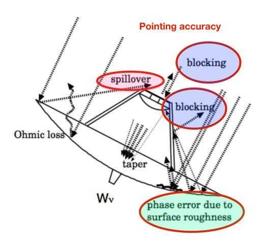
As the radio emitter moves away from the middle of the beam the angle of the waves hitting the beam changes.
