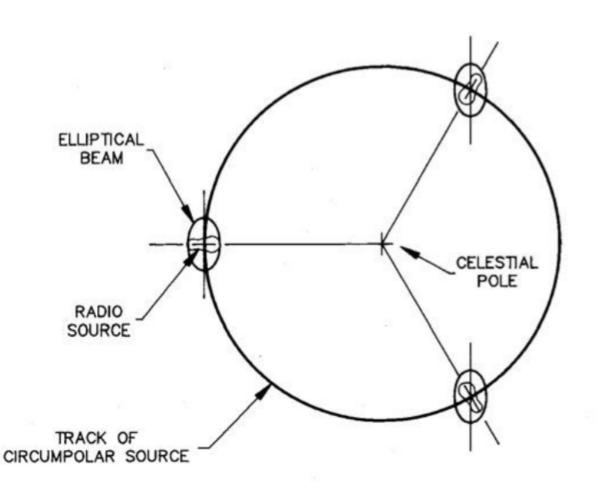
Disadvantage of alt-az telescopes is that the orientation of the telescope beam changes as the source moves across the sky.
