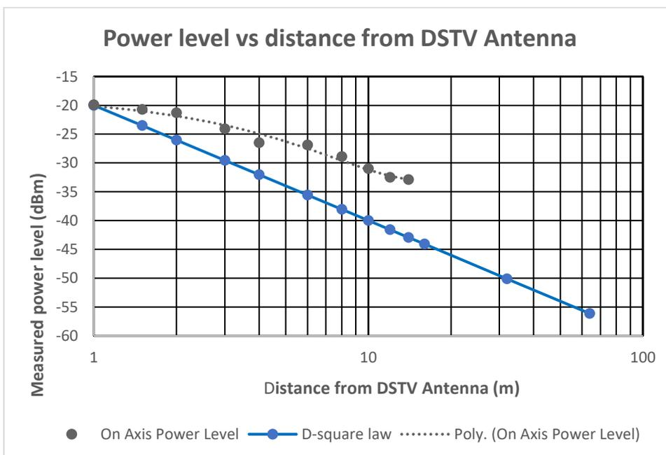
**Figure 2.** This figure shows that close to the antenna, the signal level does not decrease as a square law, but remains relatively constant for the first few metres. Only in the far field would one expect the the square law to apply, i.e. at distances  $> 14$  metres.
