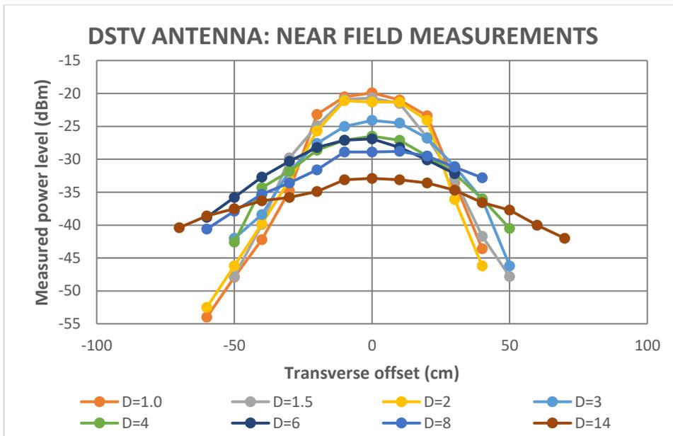
**Figure 1.** Transverse near field power measurements for 60 cm DSTV antenna. Note that within the first few metres the power does not spread, but is confined to a column known as the near field or the Fresnel diffraction zone. This zone extends typically for a distance of  $D^2/(\lambda)$  or  $2*0.6*0.6/0.025 = 28.8\text{m}$ .
