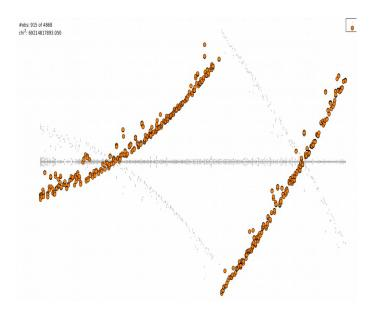
In order to select the time for the clock break we have to zoom in using the magnifying glass symbol on the upper left of the GUI. When we sufficiently zoomed in we can click the *add clock break* button and click exactly on the clock break (between observations). Click on *Yes* and the clock break is written to your OPT file.
