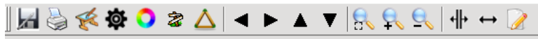
Figure 7.23: The toolbar for the Spectral Profile tool allows the user to save the spectrum, print or save the tool as an image, edit preferences (general, tool, legend), spectral smoothing, pan or zoom around the spectrum, select a range of interest, jump to a channel, or add a label.
